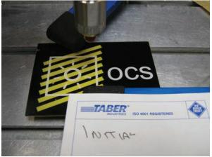
• The test was started and continued to 3600 cycles. The test was stopped and the Wearaser was refaced.
