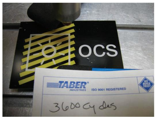
• The test was restarted and continued for an additional 3600 cycles for a total of 7200 cycles.
