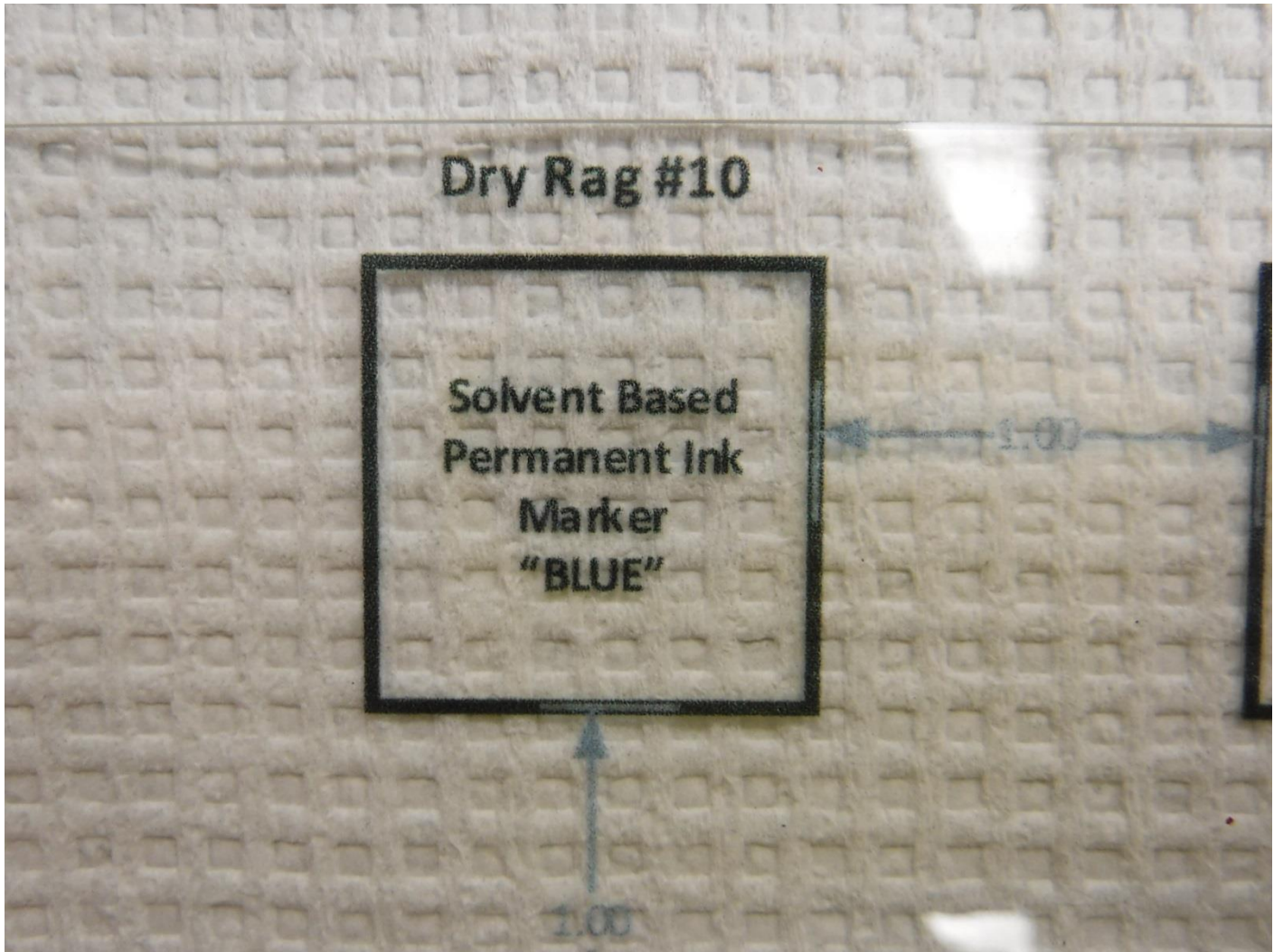
SN00006 After Test – Representative Solvent Based Ink Marker
